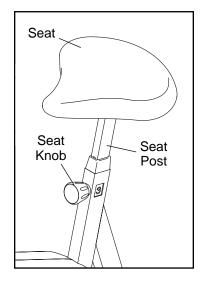
seat knob. Move the seat post up and down slightly until it locks into position. Then, tighten the seat knob. CAUTION: Make sure that the pin on the seat knob is inserted into one of the adjustment holes in the seat post. Do not rest the seat post on top of the pin on the seat knob.
